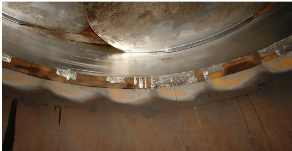
Example: Discharge ring cavitation erosion
