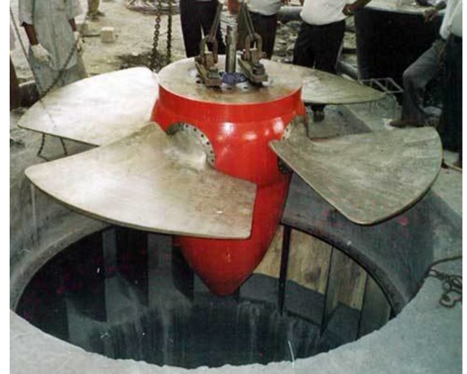
Kaplan runner: double regulated hydraulic turbine (guide vanes and blades positioning can be adjusted)
