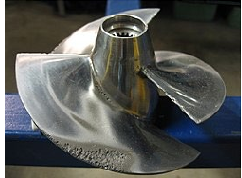
Example: Propeller with cavitation pitting erosion
