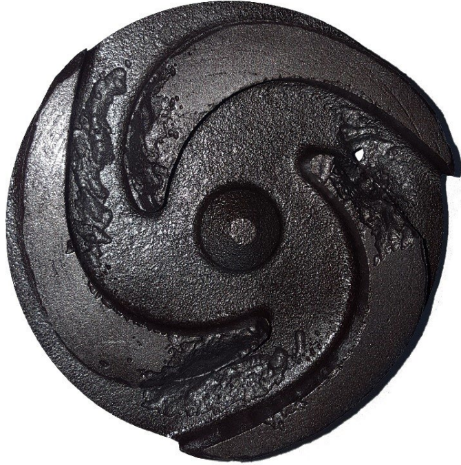
Erosion due to suction cavitation: too low pressure or setting level
