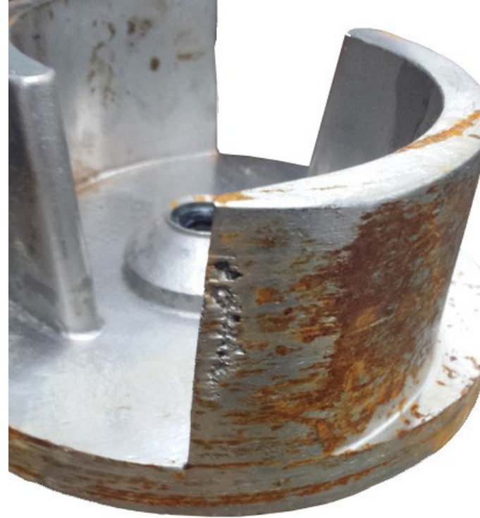
Erosion due to discharge cavitation
